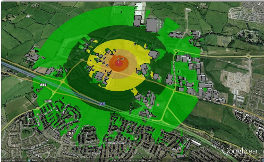
Figure 25. Overlaying a wind turbine noise prediction model on top of a Google Earth map (Source: AWNConsulting, Dublin, 2017).
