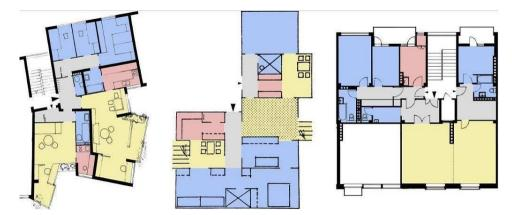
Fig. 8 Characteristic apartments with the option of unit division: 1) Siemensstadt, Berlin (Hans Scharoun, 1958) (Source: Borsi, 2018:1116); 2) Apartment "plus-minus" (concept) (Source: Mate Bajlon, 1979:51); 3) Residential building at 14 Pariska street, Belgrade (Mirko Jovanović, 1956) (Source: author's archive)
