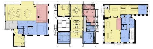
Fig. 7 Characteristic apartments with auxiliary entrance through working space: 1) Casa N, Murcia (Ad-Hoc, 2015); 2) Residential building in Senjak, Osijek (Andrija Mutnjaković, Stanka Polić, Ivan Tomičić, 1968); 3) Photographer's Loft, New York (Desai Chia Architecture, 2014) (Source: author's archive)
