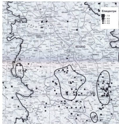
Fig. 3. The Seismological hazard map for the Kolubara region for a return period of 500 years
