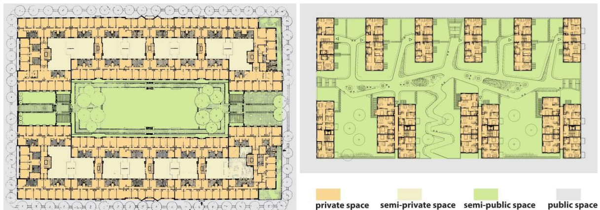
Figure 2. Experiencing territorial levels in the structure of the housing community: a) closed block (Casa de las Flores, Madrid, Secundino Zuazo, 1932) (left) and b) open block (Affordable Housing, Wroclaw, Arch_it piotr zybura, 2017) (right) (Source: author's archive)
