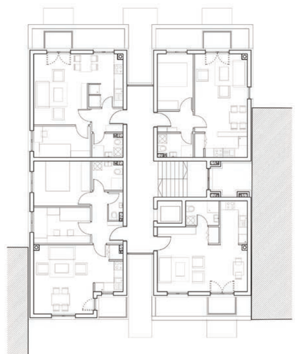
Fig. 2. Typical 1st and 2nd floor plan (left) and 3rd floor plan (right)
