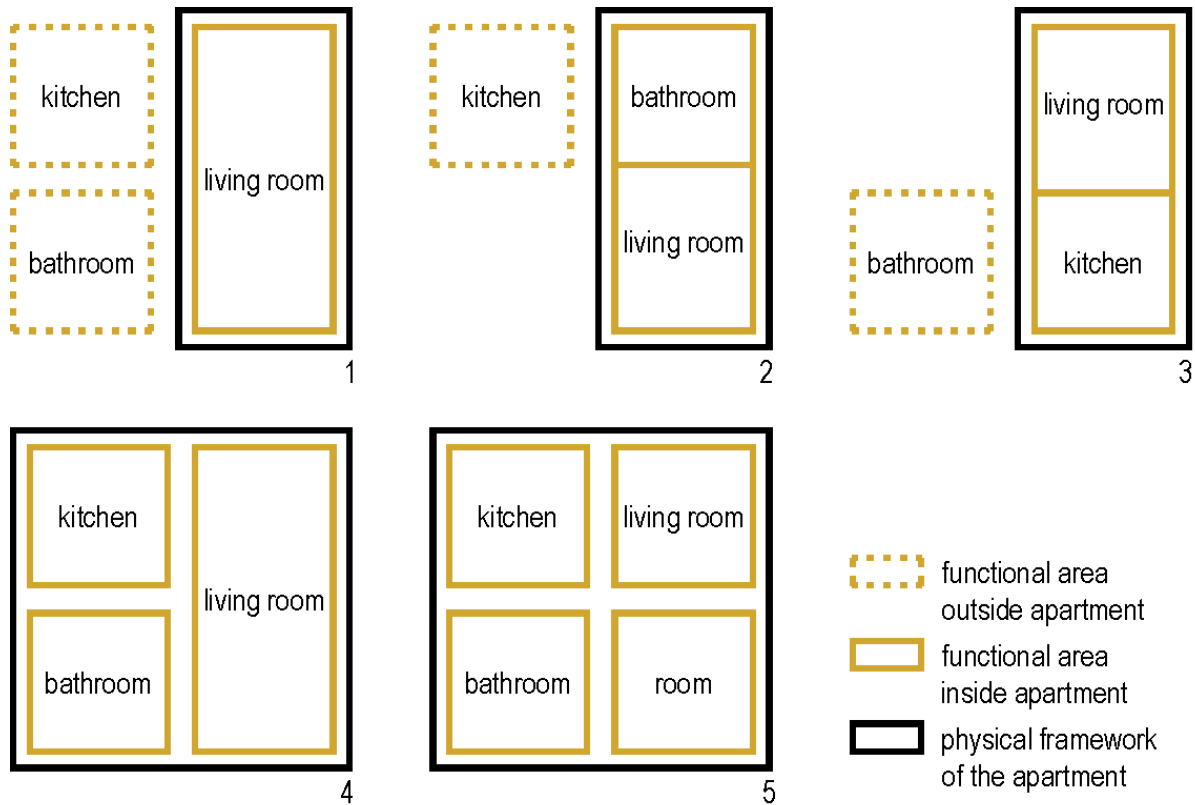
Figure 8: Typology of micro apartments according to the structure of the rooms: 1) Type 1 - [LR] + K + B, 2) Type 2 - [LR + B] + K, 3) Type 3 - [LR + K] + B, 4) Type 4 - [LR + B + K], 5) Type 5 - [LR + B + K + BR] 151 (Source: author's drawing)
